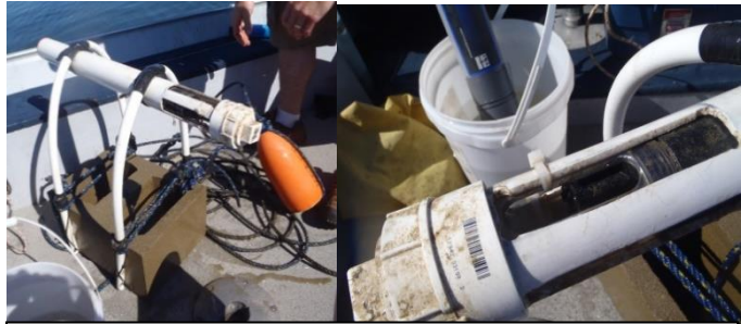
Figure 2. Sonde in protective shroud attached to a frame and concrete anchor for marine bottom deployments (left), with focus on sensor end (right).
