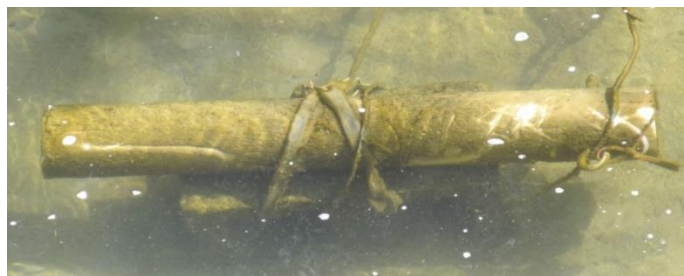
Figure 1. Algae and other fouling materials adhering to shroud and monitor. To protect monitors and reduce the need for abrasive cleaning, a shroud can be used to cover
